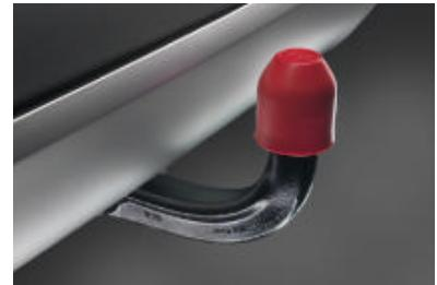
□ **Tow bar** with removable ball head (the ball head can be conveniently stowed away under the luggage compartment floor). Depending on the model, the trailer load can be up to 2,000 kg.
