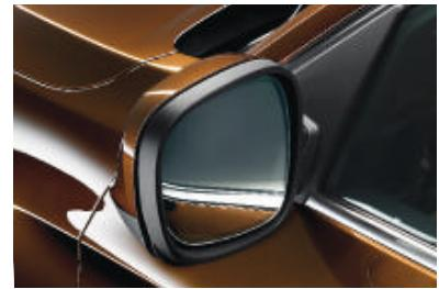
■ **Exterior mirrors**, in body colour, both electrically adjustable and aspheric on the driver's side. The mirrors can also be heated.
