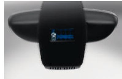
**Rain sensor, incl. automatic driving lights**: Once activated, the rain sensor automatically turns on the windscreen wipers according to the intensity of the rain and independently controls the wiper interval. The integrated automatic driving lights automatically switch to low beam at dusk or when entering tunnels.
