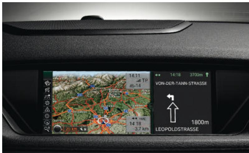
□ **Navigation system Professional\***, incl. radio BMW Professional, with DVD drive, iDrive Controller with direct menu control buttons, eight functional bookmarks, integrated hard disc for maps and audio files, fixed and high-resolution 8.8-inch graphic display, map or perspectival route display, bird's-eye view.
