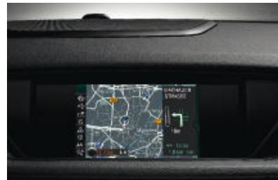
□ **Navigation system Business**, incl. CD drive, iDrive Controller with direct menu control buttons, functional bookmarks, integrated storage facility for navigation data and high-resolution 6.5-inch display.
