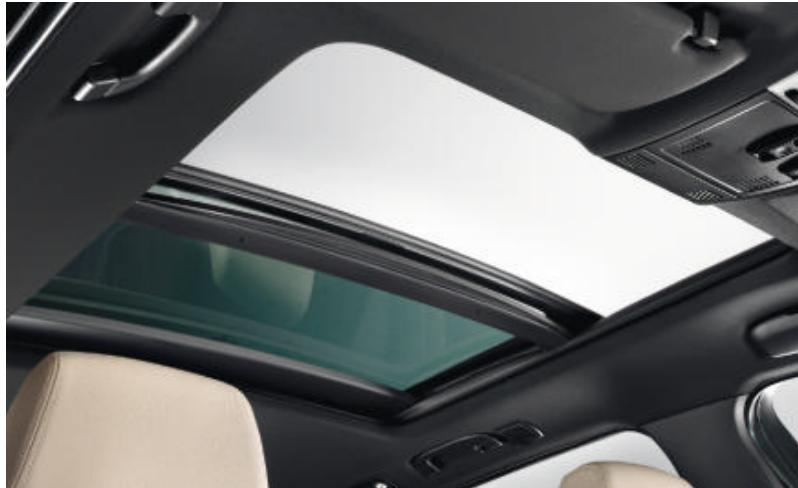
□ **Panorama glass roof** with large opening and viewing area and wind deflector. The front half of the glass can be electrically raised by touch control and also has a sliding function, electric sliding roofliner (sun protection) as well as a comfort open/close function with trap release.
