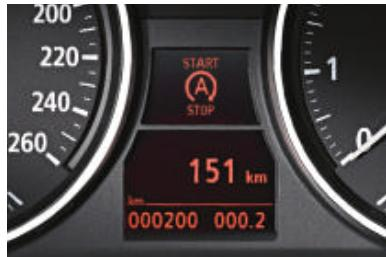
■ **Auto Start/Stop Display** signals on the Info Display when the engine has been switched off by the Auto Start/Stop function (for instance, at traffic lights or in a jam). The display is turned off when the engine is re-started automatically (for four-cylinder models in conjunction with 6-speed manual transmission).
