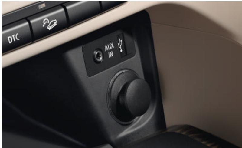
■ **AUX-IN connection**, incl. 12-V socket for an external audio source such as an MP3 player.
