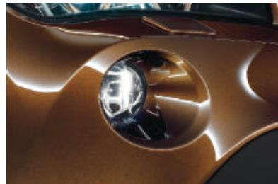
■ **Fog lights**, integrated in the front apron, for improved safety in poor visibility. Option includes heated exterior mirrors and windscreen washer nozzles.
