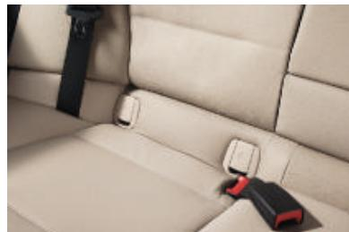
■ **ISOFIX child seat attachment**, rear on the two outer rear seats for safe attachment of a child seat with clip-in plug connectors plus additional fastening points on the upper part.
