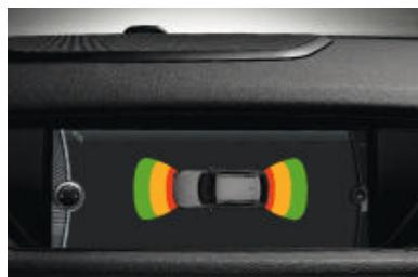
□ **Park Distance Control, front and rear**, facilitates parking and manoeuvring in confined spaces, giving an acoustic signal to indicate the distance between your car and an obstacle. In conjunction with an optionally available navigation system, the distance is also shown visually in the Control Display.
