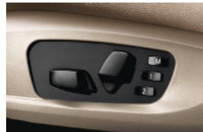
**Seat adjustment** for driver and front passenger with electric seat height and backrest adjustment, as well as fore/aft and seat angle adjustment, with memory function for driver's seat and exterior mirrors (including automatic parking function). Two personalised positions can be stored for the settings of the driver's seat and the exterior mirrors.
