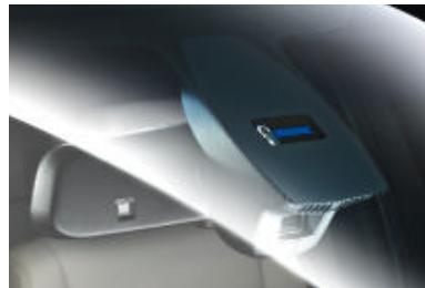
**High-beam assistant** helps the driver at night by automatically switching between high and low beam according to oncoming traffic, vehicles driving in front and when road lighting is sufficient.
