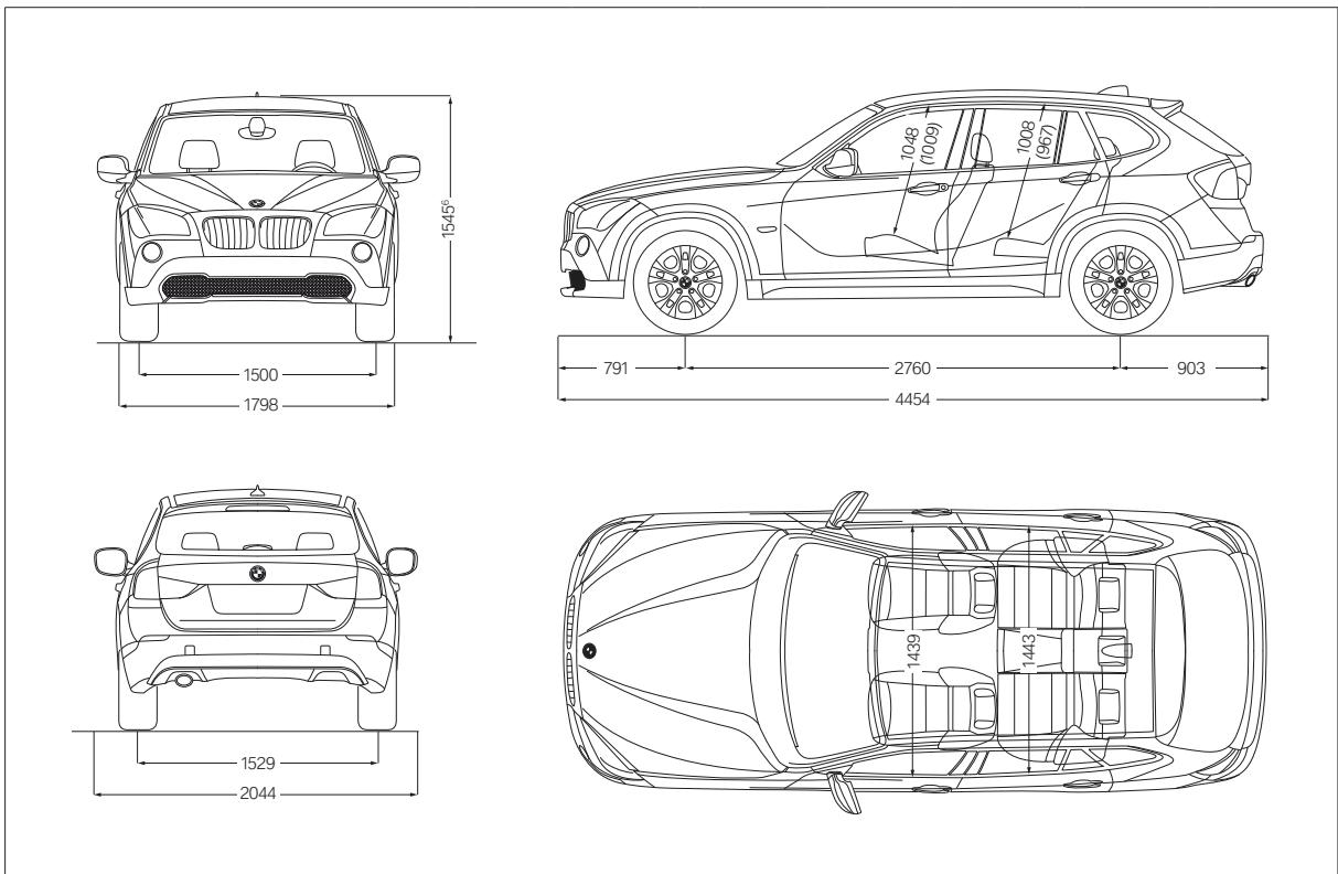
All dimensions in the technical drawings are given in millimetres. Luggage compartment volume 420 – 1,350 litres. Values in ( ) are for vehicles with panorama glass roof.
