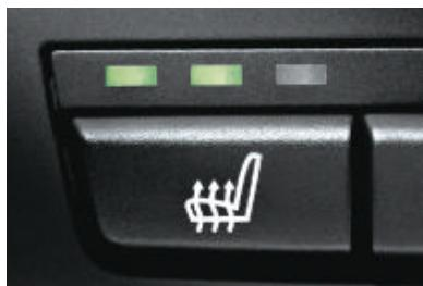
**Seat heating** (with three levels) for driver and front passenger. Seat surface and backrest, including side supports, can all be heated and deliver warmth shortly after you pull away.
