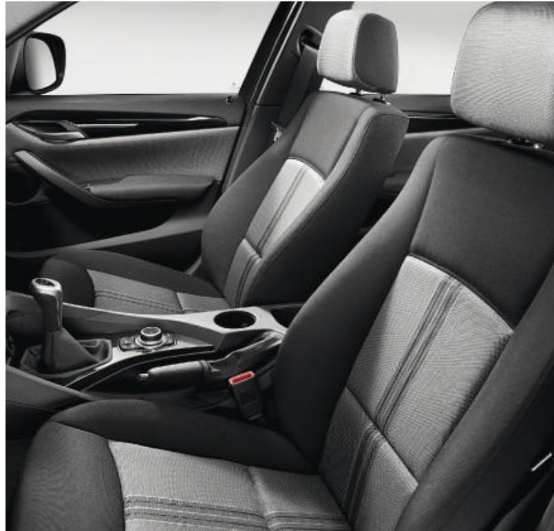
■ **Standard seats** with manual adjustment of seat height, fore/aft position, backrest angle and height of headrests.
