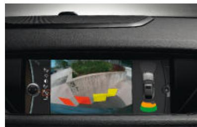
□ **Rear view camera** clearly shows the area behind the vehicle on the Control Display. Interactive guidelines indicate, for example, if a parking space is large enough for the vehicle. If the BMW has a tow bar, the image area is enlarged. The rear view camera is automatically activated when reverse gear is engaged (in conjunction with a navigation system).
