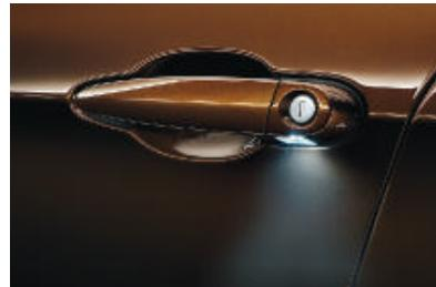
**Lights package** includes vicinity lights in the door handles, which illuminate the area outside the doors for 20 seconds when the doors are unlocked to ensure safe access in the dark. Other features include reading lights at the front and rear, footwell illumination at the front, vanity mirror lights for driver and passenger, and ambient light.
