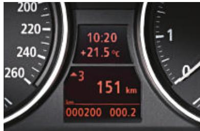
■ **On-board computer** provides information about average speed, average and current fuel consumption, range and outside temperature. ■ **Optimum Shift Indicator** lets you know when it is more economical to drive in another gear. It indicates when to shift up or down and adapts these recommendations to your driving style (for models with 6-speed manual transmission).
