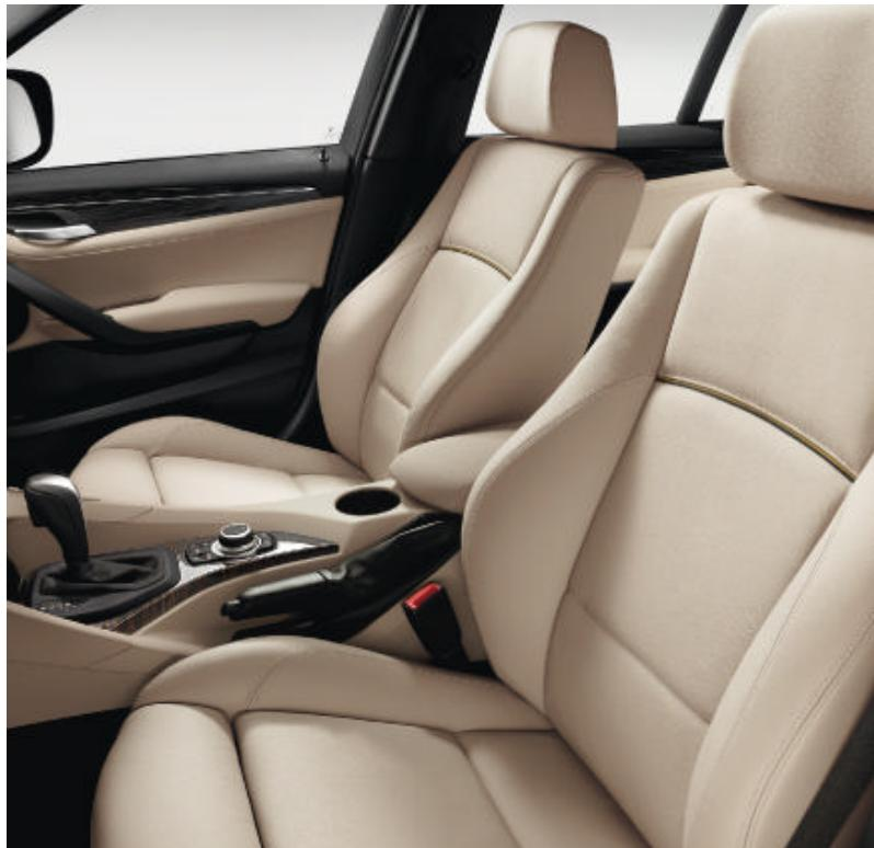
**Sports seats** for driver and front passenger, with higher seat cheeks and electric seat backrest width adjustment for optimum lateral support. Manual adjustment of fore-and-aft position, seat height, backrest angle, seat angle and thigh support.
