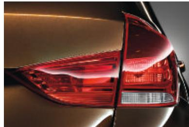
■ **Dynamic Braking Lights** help vehicles following behind to see how hard you are applying the brakes. During normal braking, the brake lights cover a large area. Only during emergency braking do the brake lights begin to flash. This allows following traffic to immediately distinguish between light braking and full braking – for even greater driving safety.
