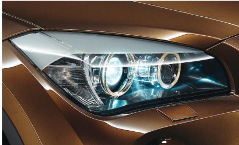
**Adaptive Headlights with variable light distribution, incl. turning lights**, only in conjunction with Xenon Headlights, optimally illuminate corners as soon as the driver turns into them through electromechanical control of the pivoting headlamps.
