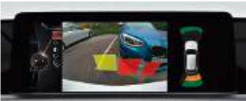
□ 3AG Reversing Assist camera 1 . Shows the area behind the vehicle in the Control Display. The rear-view camera provides a better view when reversing in parking situations at speeds below 10mph. In models with a tow bar, the Reversing Assist camera has an extra zoom function.
