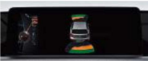
□ 507/508 Park Distance Control (PDC) front and rear or just rear, makes parking and manoeuvring in tight spaces much easier. The proximity of obstacles is indicated acoustically and visually in the Control Display.
