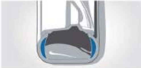
□ 258 Run-flat tyres , reinforced side walls prevent the tyres from completely collapsing or loosening from the rim if the air pressure drops. ■ Tyre Pressure Monitoring notifies the driver of any tyre issues. A minor loss in pressure is signalled by a light in the cockpit, while any greater loss is additionally signalled with an acoustic warning.
