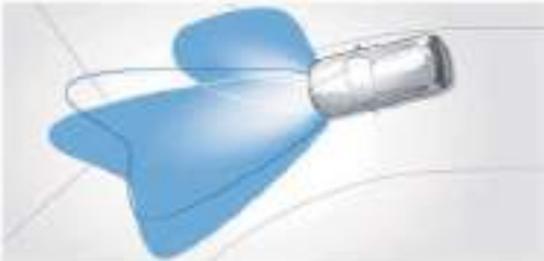
■ 524 Adaptive Headlights with variable light distribution, including cornering lights and High-beam Assistant, illuminate bends at greater distances by optimally adjusting the swivelling headlights as soon as the driver turns the steering wheel. To improve short-range visibility, the cornering lights integrated into the foglights are automatically activated, even when the vehicle is at a standstill, as soon as the indicator is switched on or the steering wheel is turned.
