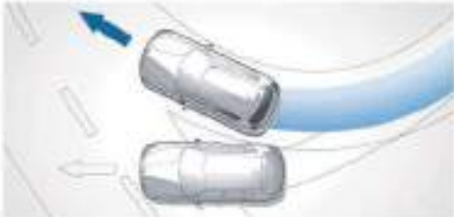
■ Dynamic Stability Control+ (DSC+) , including Cornering Brake Control (CBC), Hill-start Assistant, Brake Assist, Brake drying function and Braking readiness. DSC recognises the risk of skidding before it occurs and stabilises the car in milliseconds. The Dynamic Traction Control (DTC) allows increased wheel slip to optimise acceleration in certain driving conditions and to enable more dynamic driving.
