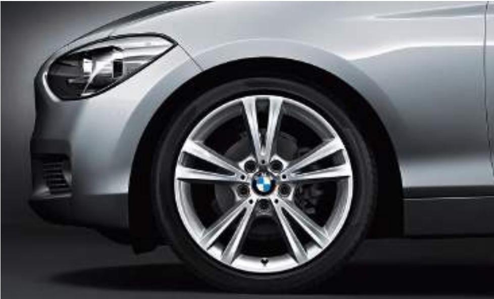
□ 2A7 18" light alloy Double-spoke style 385 with mixed tyres; front 7.5J x 18 with 225/40 R18, and rear 8.5J x 18 with 245/35 R18 run-flat tyres. (Standard with Sport Plus package).
