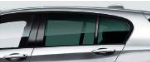
□ 420 Sun protection glass 1 prevents the interior from heating up excessively when exposed to direct sunlight, thereby ensuring a pleasant interior temperature. The more heavily tinted rear windows behind the B-pillars absorb the sunlight to a greater degree. (Standard with Sport Plus package and M Sport Plus package).
