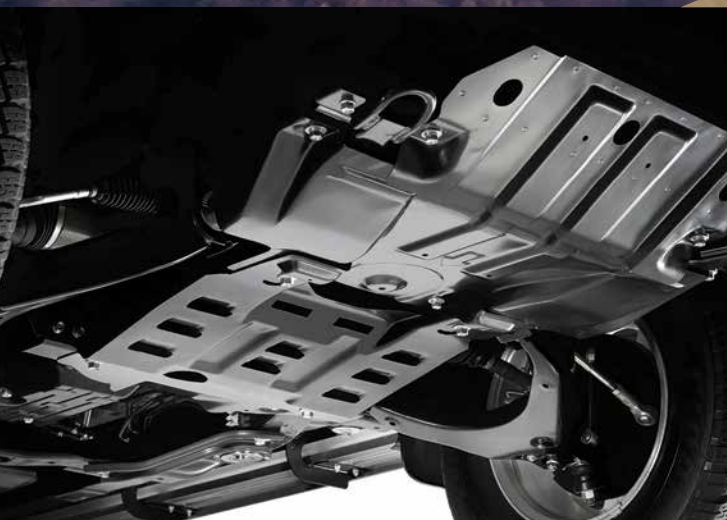
Underbody protection, front steel plate skid/shield
