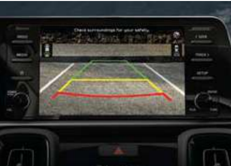
Rear View Monitor (RVM) When the transmission is in reverse, the 8-inch audio display shows the area behind the Sonet, with parking guidelines superimposed on the video image.
