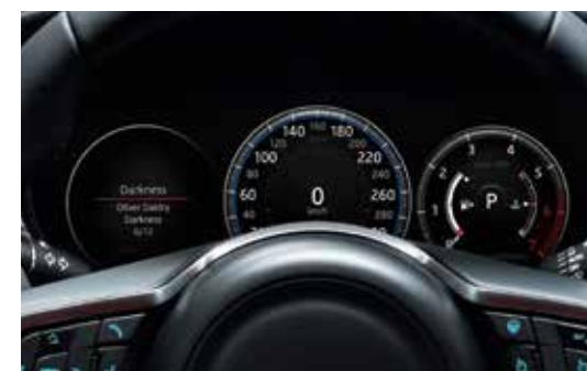
12.3" Full Digital Instrument Panel with virtual dials
