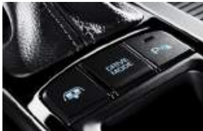
DRIVE MODE CONTROL SYSTEM This lets you choose from three different driving modes—normal, sports, and eco—depending on the steering feel you require and to suit different driving conditions.
