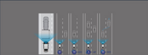
Adaptive Cruise Control(ACC) with Low-Speed Follow(LSF)
