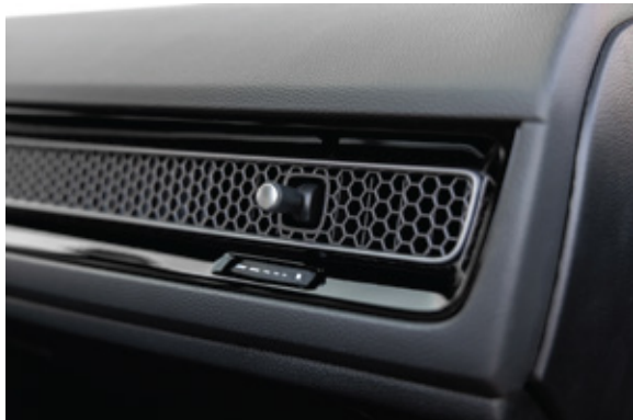
The Joystick-like Controls for The HVAC Vents Hidden Behind The Mesh
