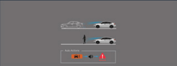
Collision Mitigation Braking System (CMBS)
