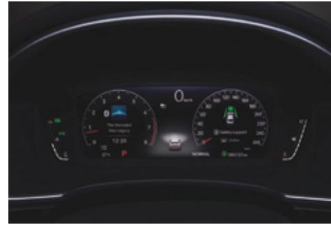
Gauge with 10.2 inch TFT Driving Information Display
